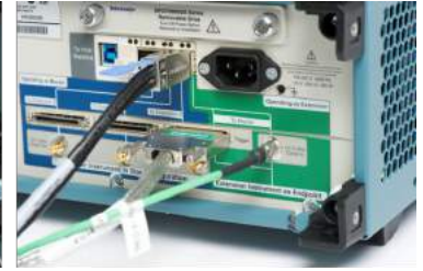
UltraSync connection on instrument with Extension role
