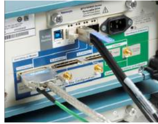
UltraSync connection on instrument with Master role
